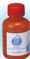
Cleaning Solution 220 (Part no. 3014028653) - contains 10% thiourea and 1% hydrochloric acid (HCl) for removing inorganic residues on sensing membrane and junction
