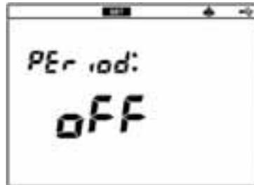
2. Press the ENTER key to enter the calibration interval change screen.
