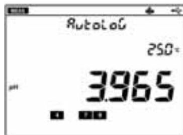
2. Press the ENTER key. "Auto LOGGING" is displayed on the screen, and the auto data memory function starts.
