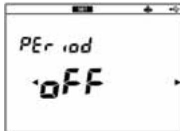
3. Press the ◀ or ▶ key to change ON or OFF, and press the ENTER key.
