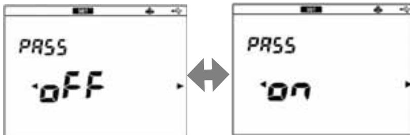
6. If you select ON, press the ◀ or ▶ key to select a digit and press the ▲ or ▼ key to change the value, and then press the ENTER key and press the ENTER key to return to the password change screen.
