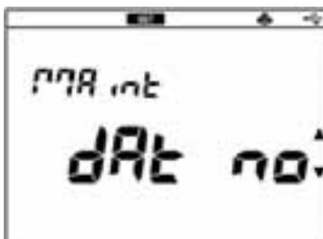
4. Press the ENTER key to display the number of the memory data currently saved in the instrument.
