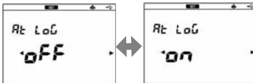
4. If you select ON, press the ◀ or ▶ key to select a digit and press the ▲ or ▼ key to change the value, and then press the ENTER key.
