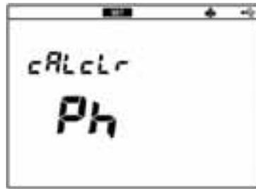
5. Press the ENTER key to enter the calibration data deleting (Yes/No) screen.
