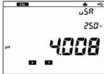
The **4** mark, which means that the pH4 calibration is completed, is displayed on the screen.
