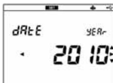
5. Press the ◀ or ▶ key to select a digit and press the ▲ or ▼ key to change the value for month and day setting, and then press the ENTER key.
