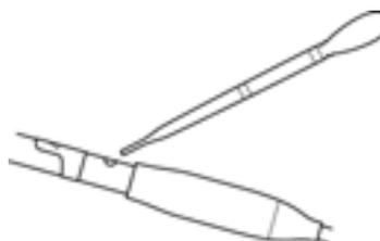
4. Fill the electrode with new internal solution (model 300), until it nearly reaches the filler port.
