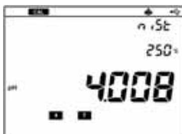
The **4** mark, which means that the pH4 calibration is completed, is displayed on the screen.
