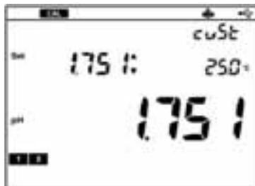
The **2** mark, which means that the second point calibration is completed, is displayed on the screen.
