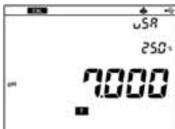
The **7** mark, which means that the pH7 calibration is completed, is displayed on the screen.
