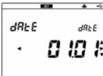
6. Press the ◀ or ▶ key to select a digit and press the ▲ or ▼ key to change the value for hour and minute setting, and press the ENTER key to return to the date setting screen.
