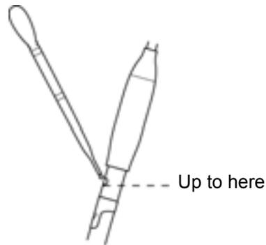
5. Wash the tip of the electrode well with pure water (deionized) and wipe it with filter or tissue paper.
