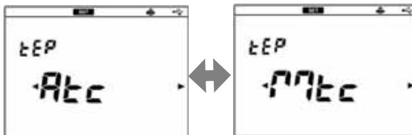
4. If you select MTC, press the ◀ or ▶ key to select a digit and press the ▲ or ▼ key to change the value, and then press the ENTER key.
