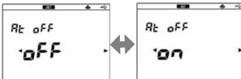
6. Press the ◀ or ▶ key to select a digit and press the ▲ or ▼ key to change the value, and then press the ENTER key to return to the auto power off change screen.
