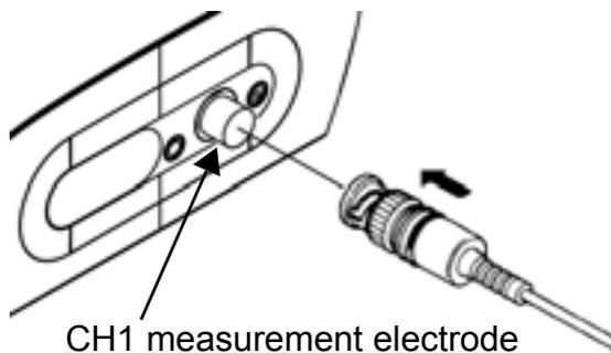
2. Turn the electrode connector to the right along the groove to plug the connector.
