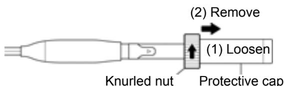
3. Open the internal solution filler port, then use a dropper to remove the internal solution.
