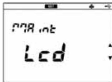
3. Press the ▲ or ▼ key to enter the temperature calibration screen.
