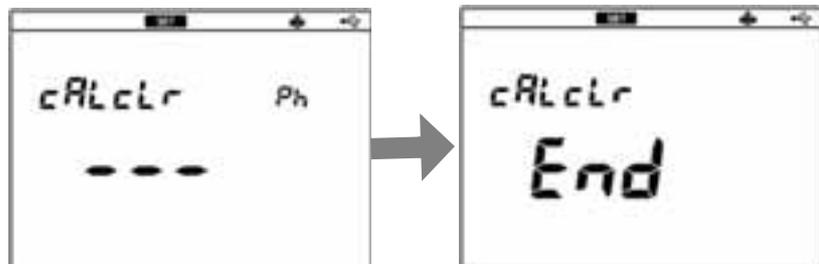
7. Press the ENTER key to return to the calibration data clear screen.
