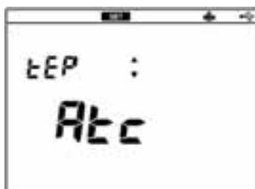
2. Press the ENTER key to enter the temperature compensation function change screen.
