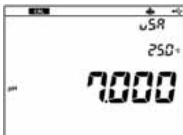
5. Check the stable indication value, and press the CAL key.
