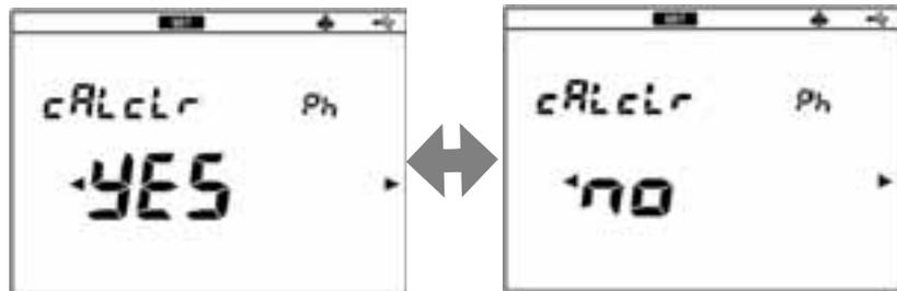
6. Press the ◀ or ▶ key to select Yes, and press ENTER key to delete the calibration data.
